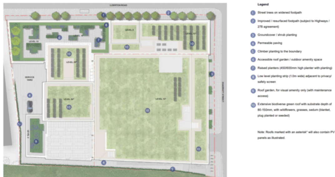
Image 34 (above): Roof plan showing the landscaping arrangement
